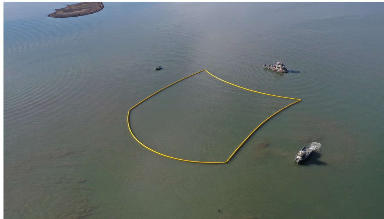
Picture shows an actual R-30 deployment in the summer of 2020. Note that the boom is not required to form a perfect diamond shape. Tide, current and winds will affect the boom shape. Anchors may need to be added or moved to ensure the boom is effective in corralling and containing the oil during changing conditions.
