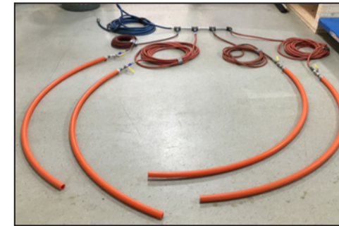
Example of multiple air lines connected to manifold to create a bubble ring. Flexible air line is attached to hard plastic pipe which is pushed under the ice through auger holes. Using rubber grommets or gaskets around the hard plastic pipe can help hold the pipes in the auger holes.
